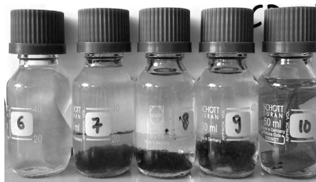
Fig. 3. Cellulose carbamate fabrics (ca. 0.5 g) in aqueous sodium hydroxide solutions (ca. 50 ml) with various concentrations (6) 0.5 M, (7) 1.5 M, (8) 2.5 M, (9) 3.5 M and (10) 5.0 M.
